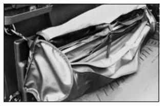
Stow both bows and the front and rear rails in the storage bag. When all components of the tonneau cover are secured in the bag properly, zip the bag shut.
